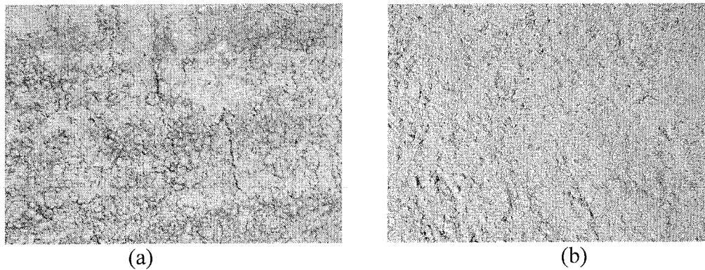
Figure 4: Asphalt Compacted by (a) Steel Drum Roller and (b) AMIR Roller
