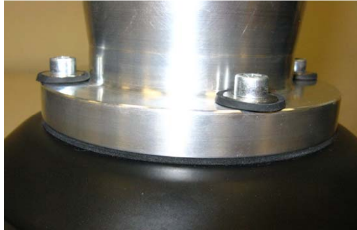
Figure 3 – Details of vibration damping rubber between compression driver and diameter matching component.
