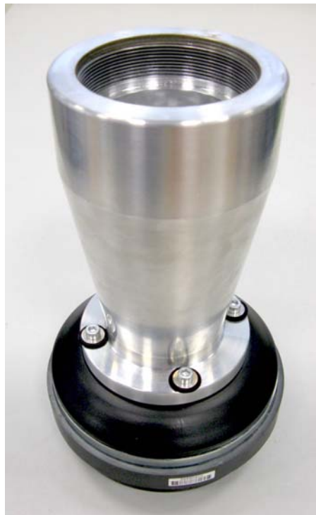
Figure 4 – Diameter matching between compression driver and principal tube.
