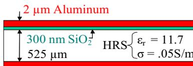
Fig. 2: Cross-sectional view of the realized patch antenna with HRS substrate.
