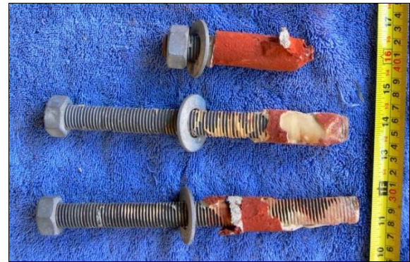
Figure 29: Recovered adhesive anchors that performed inadequately.
