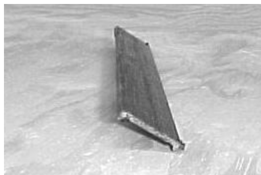
Fig. 7 – U-Shaped pultruded profile
