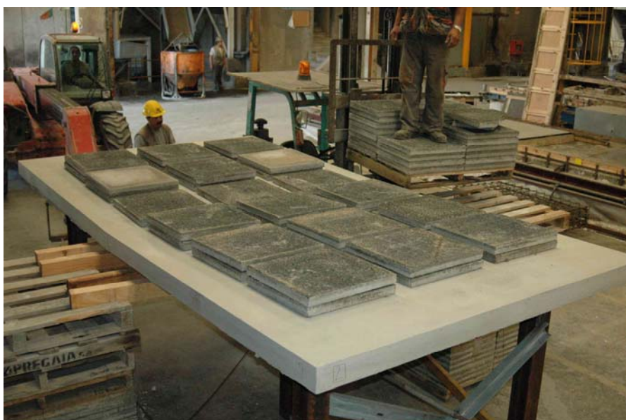
Fig. 5.5 - Final view of the panel, loaded with 33 concrete plates.
