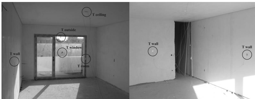
Figure 4: Schematic view of instrumentation placed (reference west room).
