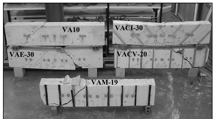
Figure 8. Appearance of the beams of series A after testing.
