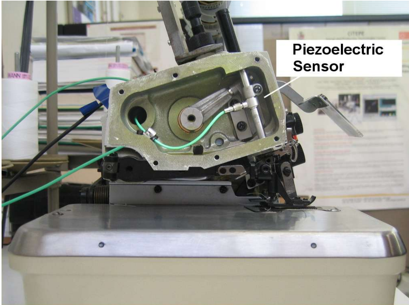
Figure 3: Set-up of the sensor for needle penetration force measurement
