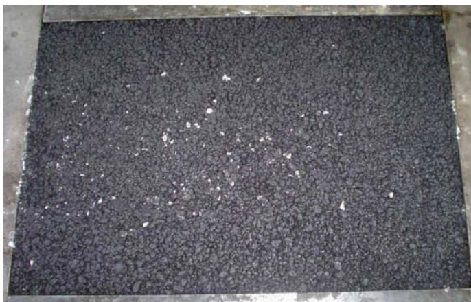
(c) laje compactada no molde
