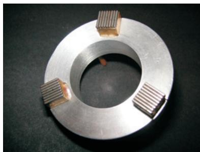
**Figure 2** (A) FRICTORQ II; (B) the upper body (or contact sensor) with three small pads, disposed at 120°.
