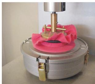
**Figure 1** (A) Geometry of the first adopted theoretical model for the FRICTORQ I; (B) first developed FRICTORQ set-up showing a detailed view of the positioning and tightening fabric clamps.
