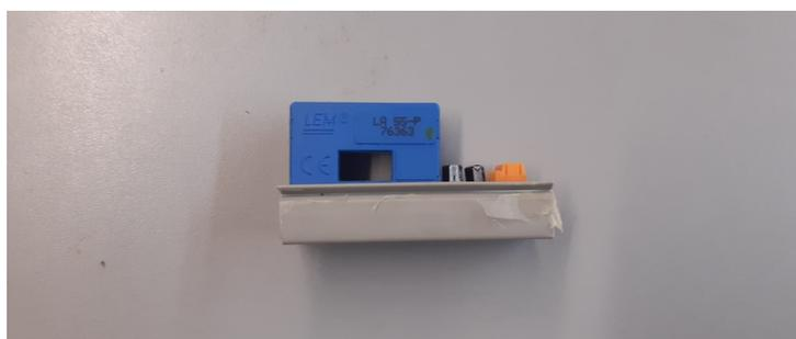
**Figure 5.6:** Sensor de corrente LA-55P.
