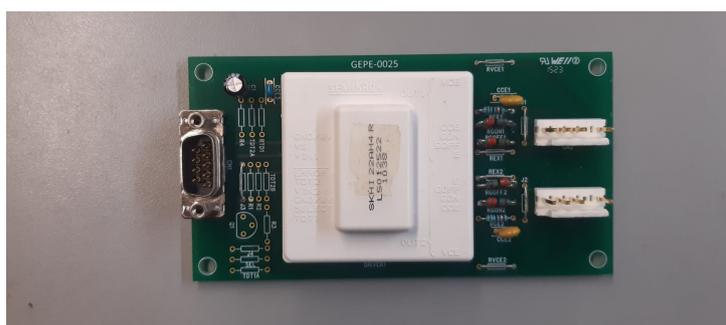
**Figure 5.10:** Circuito de *drive* dos IGBT.
