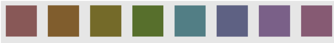
Figure 80 - sRGB computational representation of samples S 5030-R and S 6030-Y40R, S 6030-Y, S 5540-G40Y, S 5030-B50G, S 6020-R70B and S 5030-R50B, S5030-R30B (from left to right).
