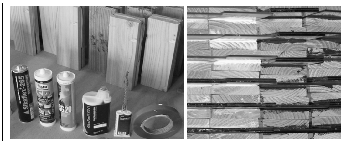
Figures 1 and 2: Adhesives and specimens used in the set of experimental tests
