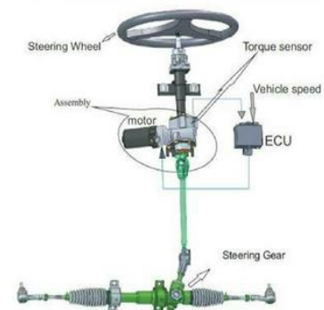
Figure 2-5c: Electric power steering [55]
