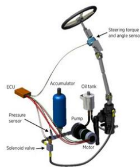
Figure 2-5b: Hydraulic power steering [55]
