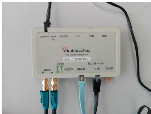
(a) The Autotalks PANGAEA V2X Communication Module
