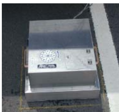
Figura 5.7 – CTMeter [Prowell and Hanson, 2005]
