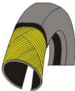
Figura 6.4 – Pneu diagonal [www.braziltires.com]
