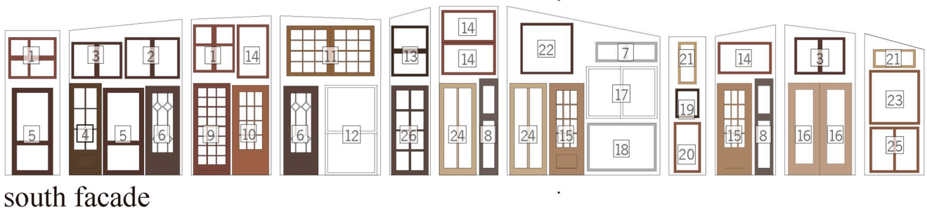
Fig. 2. Reused window frames in south facade and vertical section of the Case Study House.
