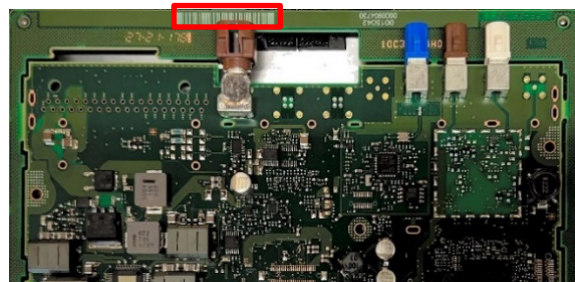
Figure 7: Example of a barcode in a PCB.
