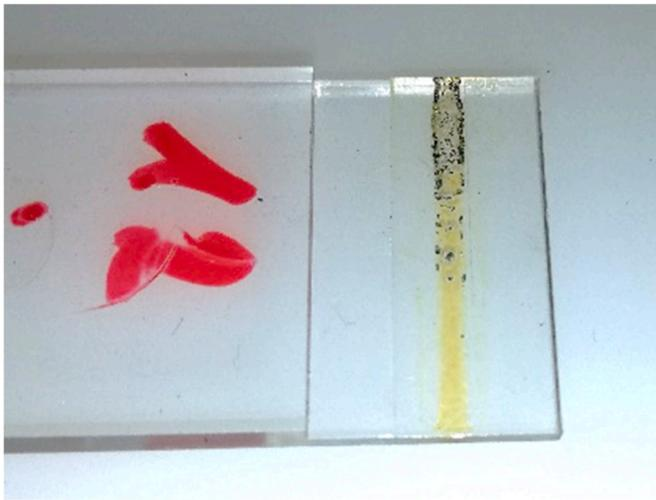
Fig. 5. PMMA burnt in samples welded at 350 °C.
