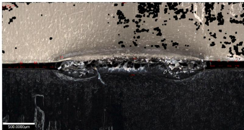
Fig. 11. Microscopic image from the side of the sample that resulted in the highest strength of the joint (triangular rib with 1.2 mm width and 0.5 mm height).
