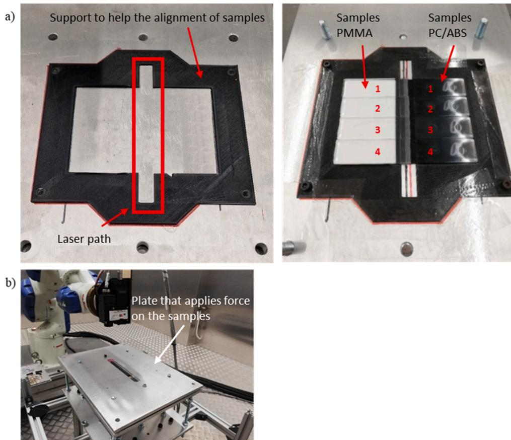
**Fig. 2.** Welding process experimental set-up: a) alignment of the samples; b) application of clamp force.
