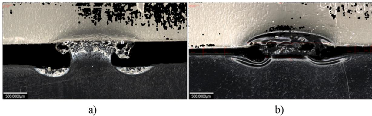
Fig. 7. Microscopic image of the side view of the sample with rectangular rib with 0.8 mm width and height welded with non-optimized (a) and best set of parameters (b).
