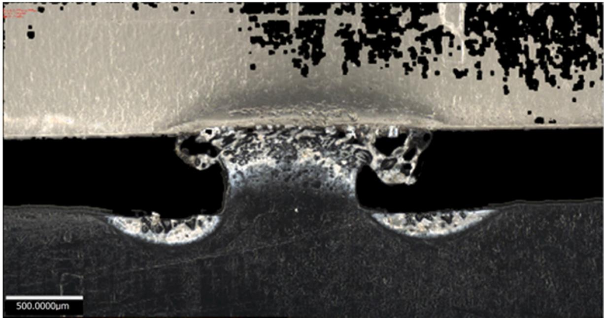
Fig. 3. Microscopic image from side of a welded sample with rectangular rib.
