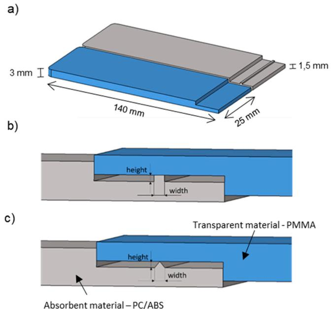
**Fig. 1.** Samples for welding: a) PMMA (blue) and PC/ABS (grey); b) PC/ABS sample with rectangular section of the rib; c) PC/ABS sample with triangular section of the rib.
