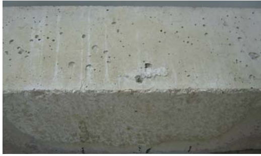
Fig.6: No spalling of beam PP 1 after 600 °C
