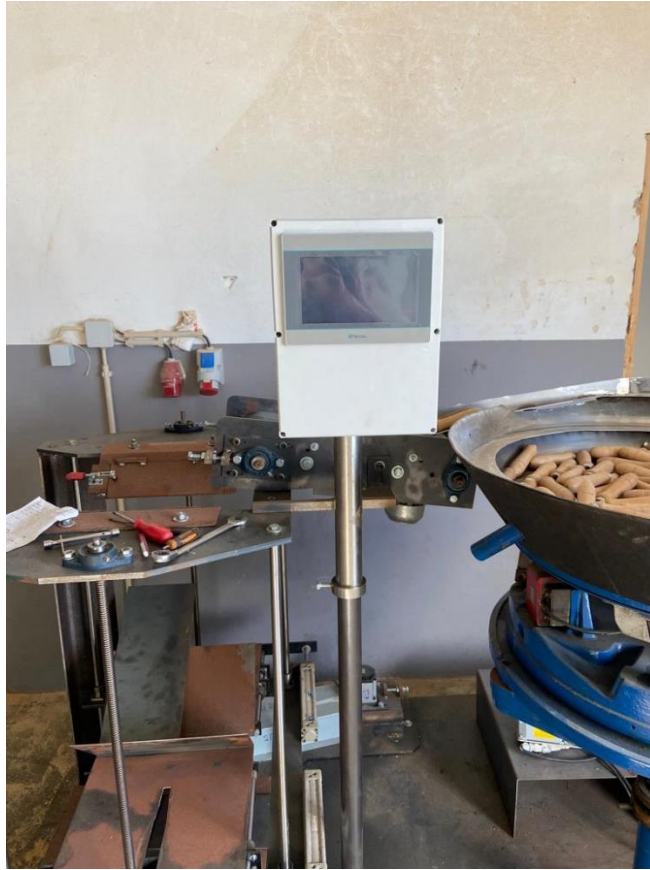
Figura 107 - Consola HMI 7" WECON Portugal
