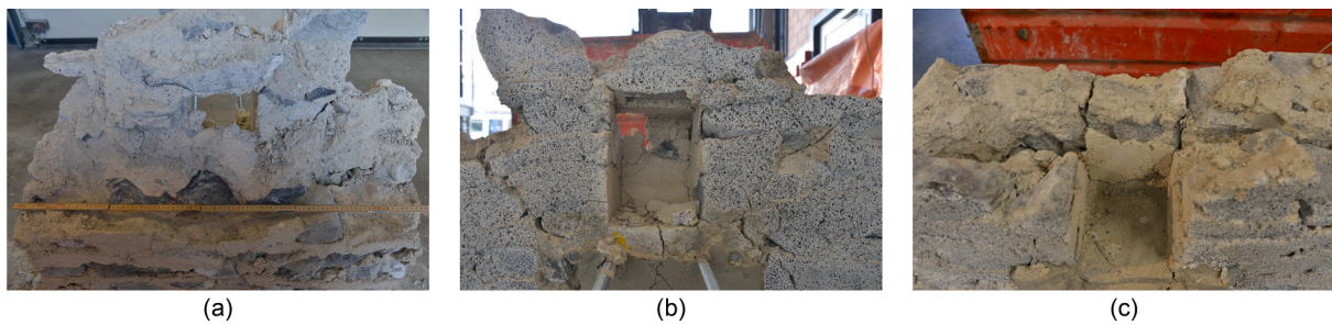
Fig. 16. Common features observed for PAT specimens: (a) top view of the breakout failure (PAT2); (b) damage at the joist pocket (PAT2); (c) cracks behind the joist pocket (PAT4).
