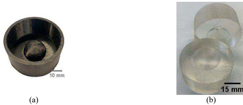
Fig. 3. A) 3d printed mold to perform the PDMS gravity casting process; b) PDMS cell to measure the NFs thermal conductivity.
