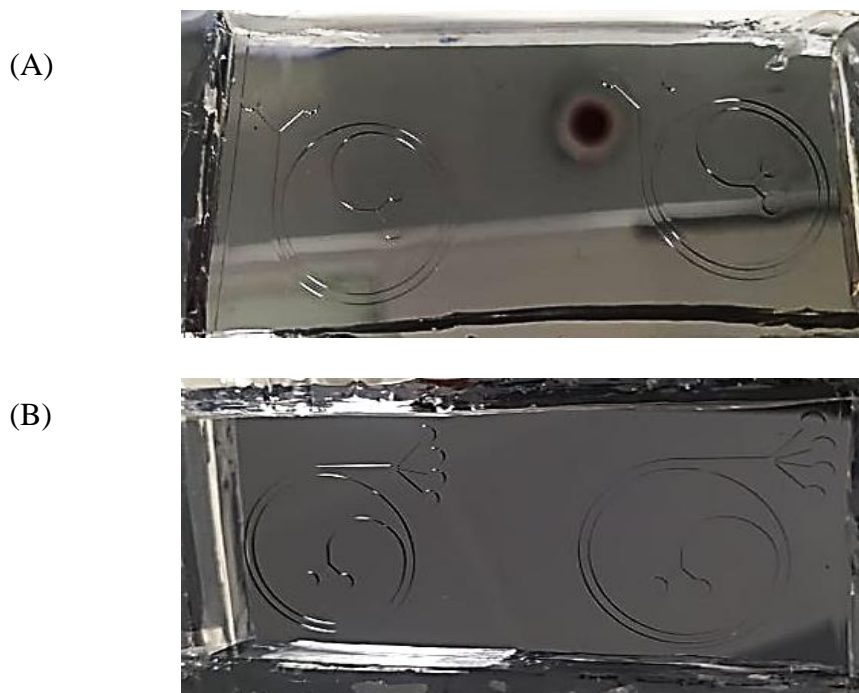
Figure 13- Silicon wafer with the devices moulds fabricated by photolithography: (A) device with two inlets and two outlets; (B) device with two inlets and four outlets.
