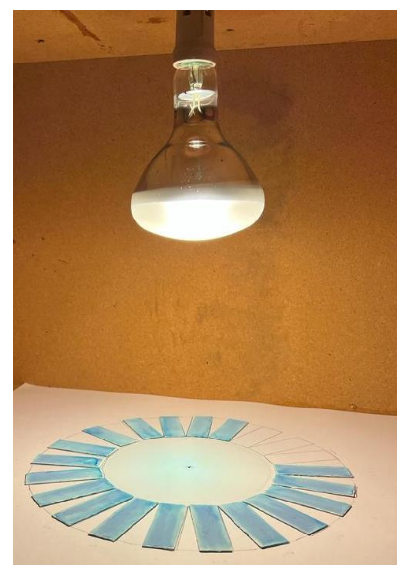
Figure 8. Setup for pollutant (Methylene Blue) degradation
