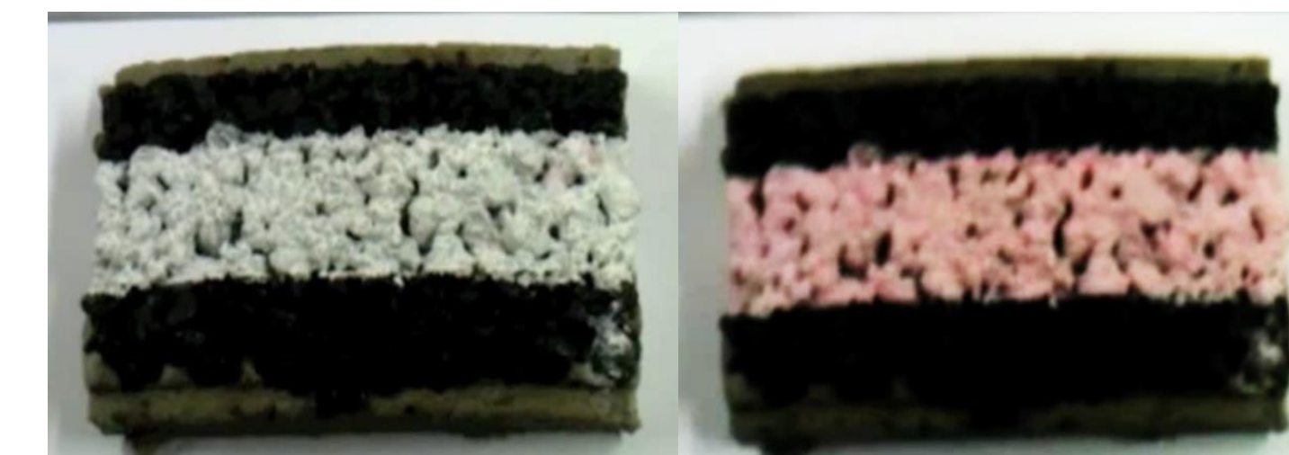
Figure 15. Thermochromic road paint sample at 25 °C (left) and 1 °C (right)
