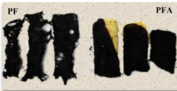
Fig. 7 Pictures of both PUR foams, PF and PFA, after flammability tests
