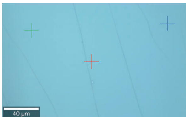
Figure 107: Measured section of oxygen plasma-treated flat PDMS. Crosses are measured spots.
