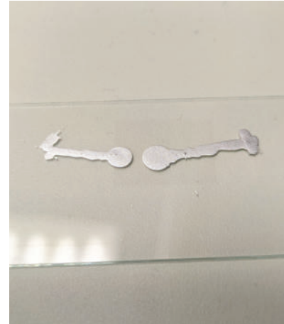
Figure 51: Conductive silver ink contacts implementation on graphene on glass.
