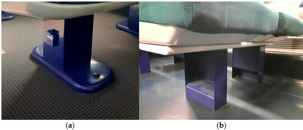
Figure 15. Seat metallic structural frame: (a) comfort seat structural frame; (b) standard seat structural frame.
