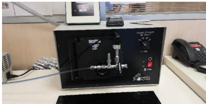
Figure 17 – Plasma Cleaner used to bond the PODMS devices with the Glass slides (Harrick Plasma Inc)
