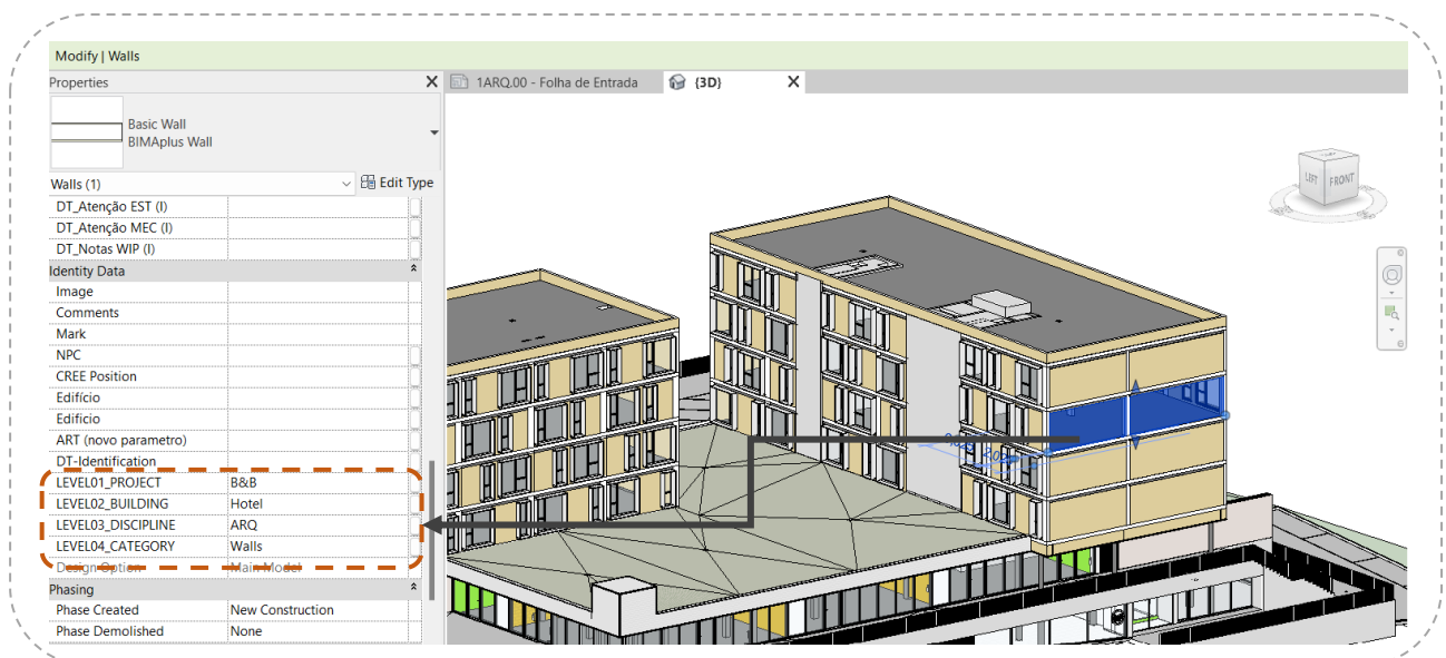
Figure 50 – Level of information need for the exterior wall on the case study, in Autodesk Revit.
