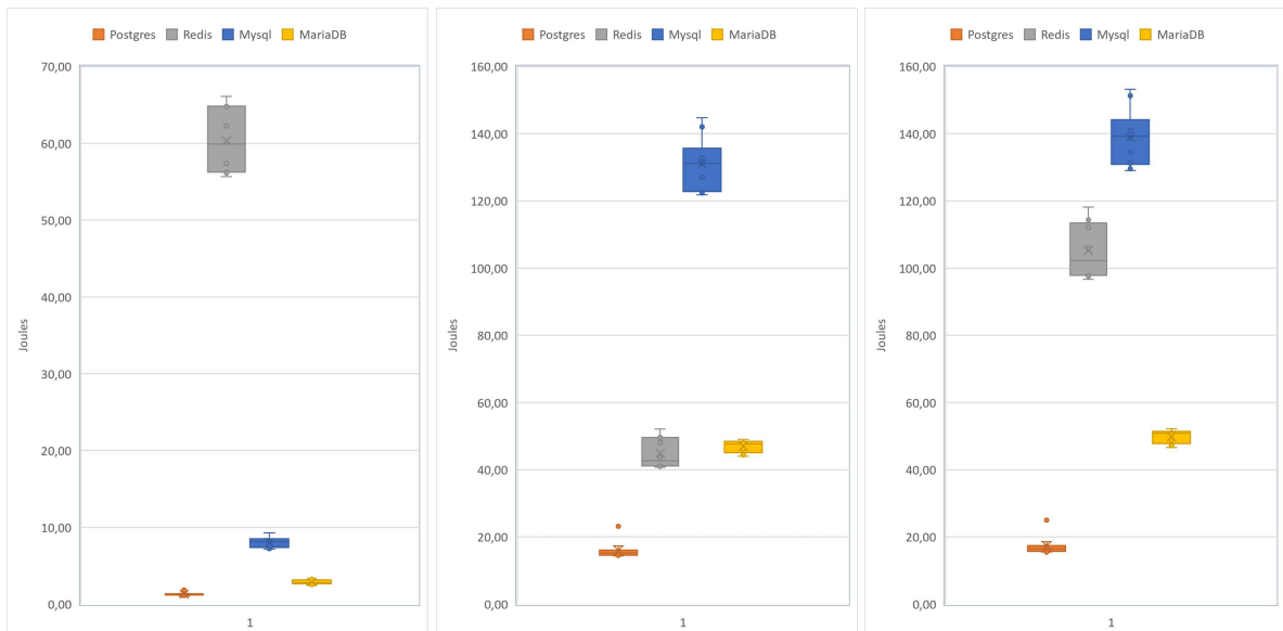
(a) Energy consumption on Package per NOPM (b) Energy consumption on Disk per NOPM (c) Energy consumption on Overall System per NOPM
