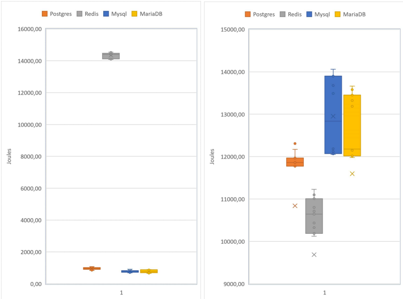
(a) Distribution of energy consumed on Package (b) Distribution of energy consumed on Disk
