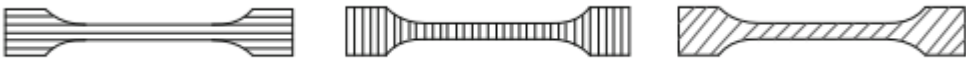
Figure 16 - Deposited toolpath pattern on the specimen in X, Y and 45° direction, respectively [53]
