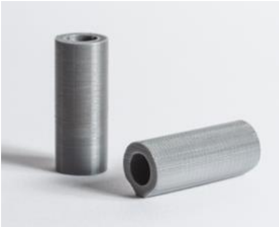
Figure 17 - Two identical cylinders printed at the same layer height in different orientations (left: vertically, right: horizontally) [54]
