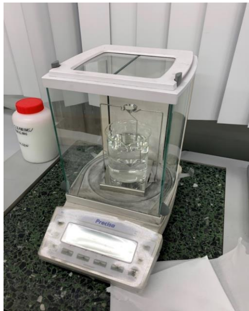
Figure 64 - Density measurements with the immersion method
