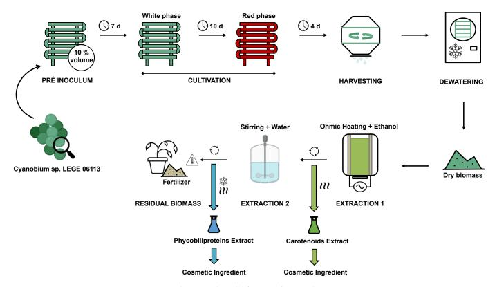
Figure 3. Final proposed model for Cyanobium sp. bioprocess.
