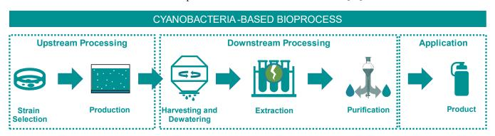
Figure 1. Overview of a general cyanobacteria-based bioprocess.
