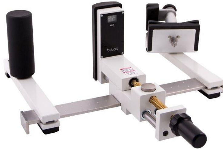
Figure 14- Telos Stress Device. (Adapted from [57])
