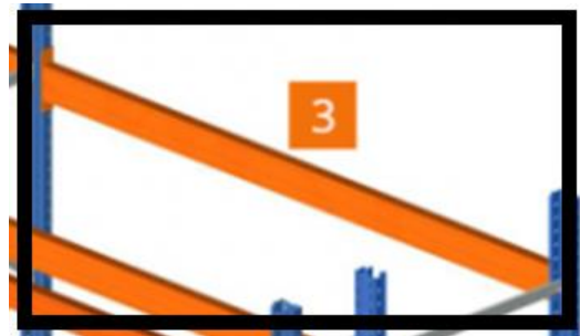
Figura 1.5 - Detalhe - Viga horizontal (Stow-Group, 2022)
