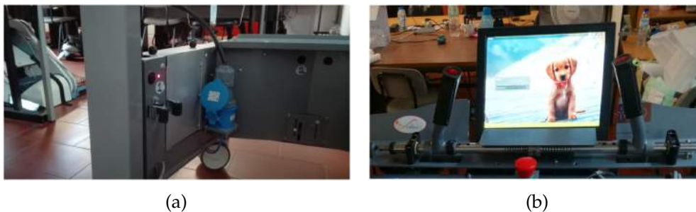
Figure 148: Starting the ASBGo* : (a) Connect the male power plug connector of the system to the battery, turn the system ON using the switch (represented as '1') and turn the on-board computer on using its power button (represented as '2'); (b) Login.
