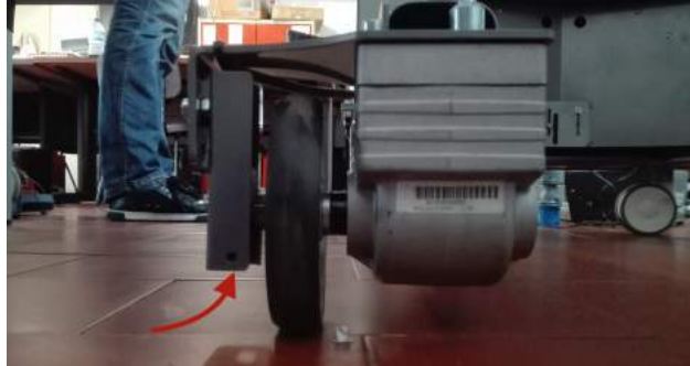
Figure 118: Encoder coupled to the left motor.
