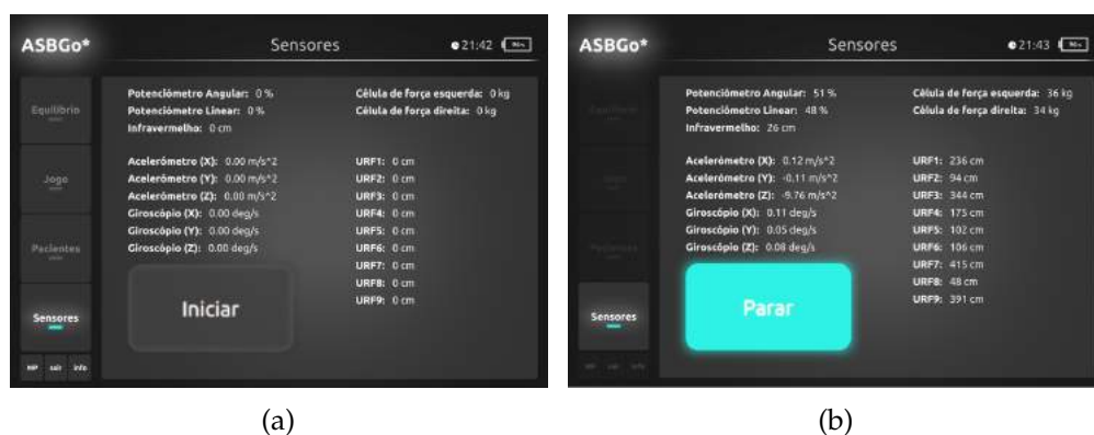
Figure 142: Local GUI 'Sensores' page: (a) Idle state; (b) Running state.
