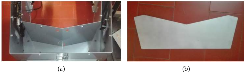
Figure 110: (a) Walker's compartment with the PCBs on the left side and the motors' drivers on the right side; (b) Mechanical piece that allows to divide the walker's compartment in floors.
