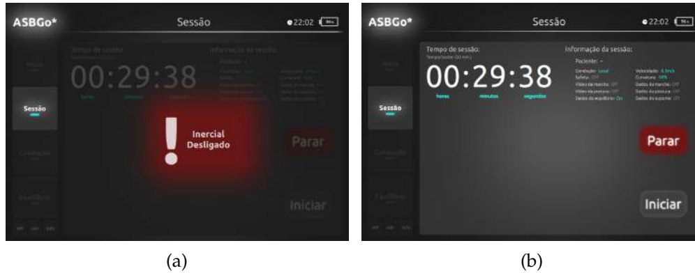
Figure 143: Local GUI IMU's warning: (a) Warning triggered pausing the session; (b) Warning disappears and session remains paused.
