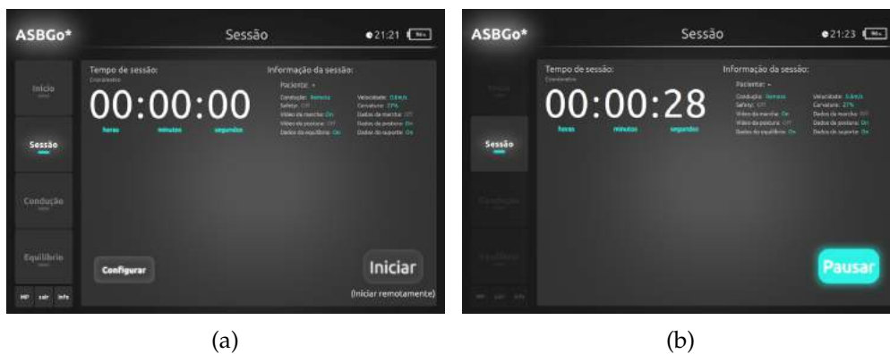
Figure 138: Local GUI session page with remote drive mode and 'chronometer' mode: (a) Idle state; (b) Running state.
