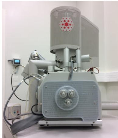
Figure 3.11: The FEI Quanta 650 FEG of the INL - International Iberian Nanotechnology Laboratory.
