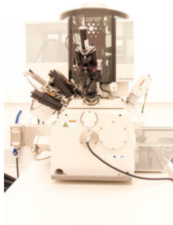
Figure 3.12: The FEI Helios G2 NanoLab 450S of the INL - International Iberian Nanotechnology Laboratory.
