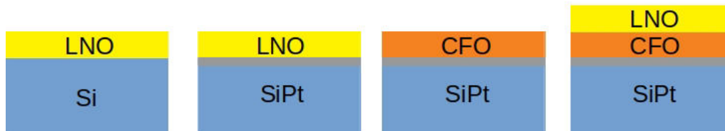
Figure 2.7: The composite systems investigated in the present study: LNO thin film on Si substrate, LNO thin film on SiPt substrate, CFO thin film on SiPt substrate and CFO/LNO bilayer film on SiPt substrate. The grey layer on the SiPt substrates represents the Pt.
