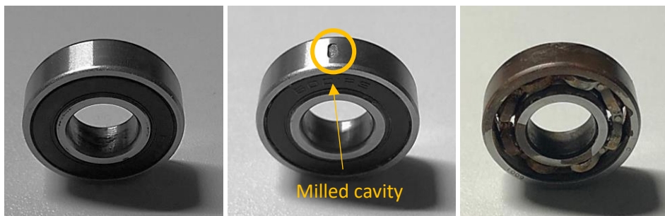
Figure 18 – New bearing, milled bearing and corrosive bearing
