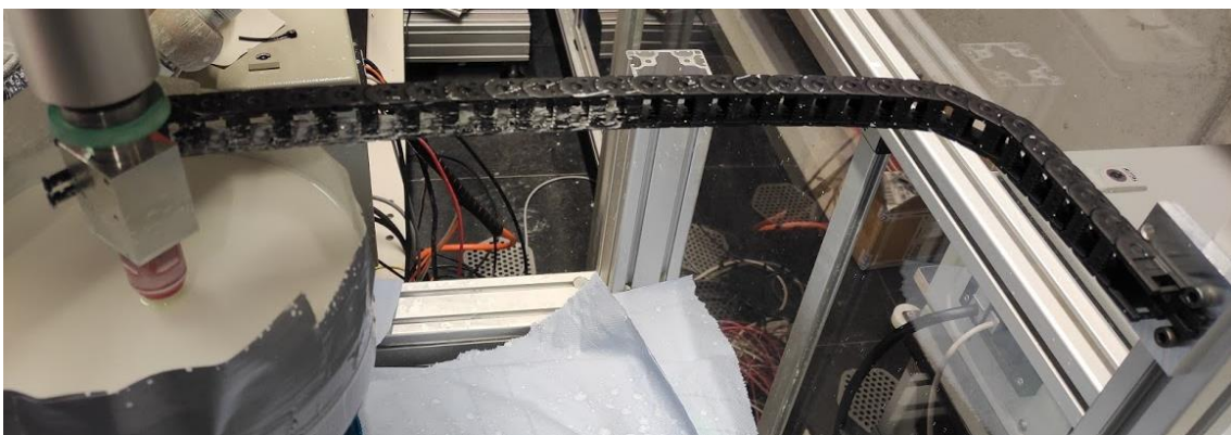
Figure 43 – Energy chain assembled into the polishing head robot
