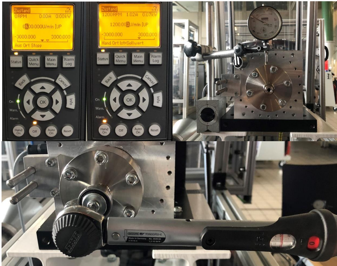
Figure 22 – Testbench controller; adapter being set-up
