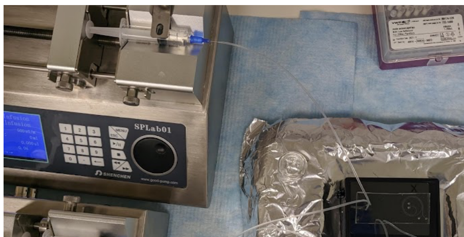
Figure 4.3 - Pumping of a filtered sample of Pluronic F-127 (Sigma Aldrich) at 1% (w/v) in PBS to the spiral chip at a flow rate of 250 \mu\text{L}/\text{min} for around five minutes, in order to get rid of persisting air bubbles within the system and to guarantee that the device's channels are hydrophobic.
