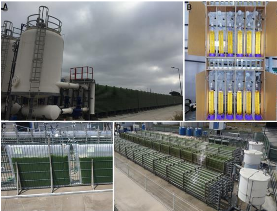
Figure 4– Different closed system production of the microalgae biomass; A: Industrial Tubular Photobioreactor; B: Bubble Column Reactors in laboratory scale; C: Flat Panel Photobioreactor; D: Tubular Photobioreactor in pilot scale. Pictures were kindly provided by Allmicroalgae, Pataias, Portugal.
