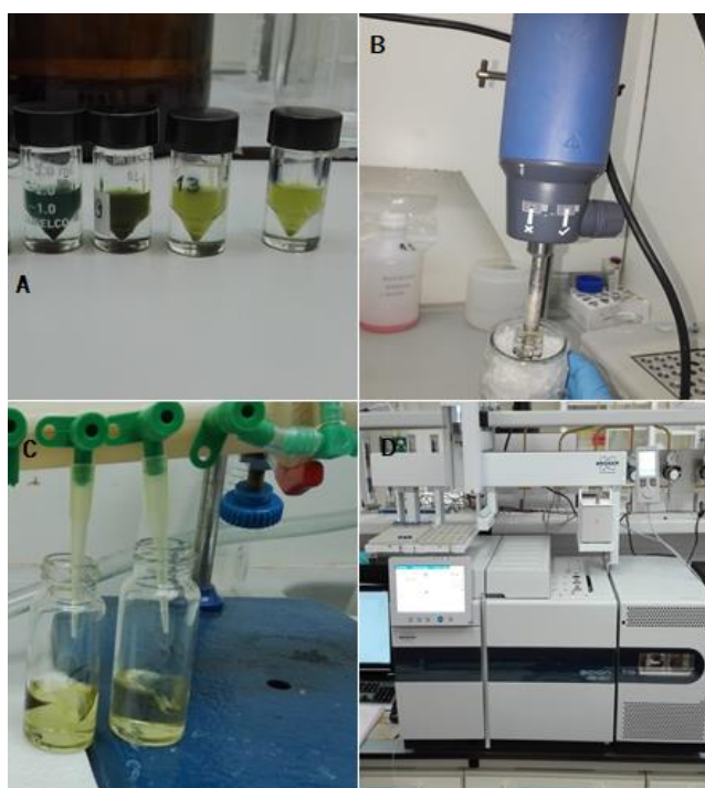
Figure 12– Different steps on FAME determination. A: Derivation vessels before homogenization with Ultra Turrax (lyophilized biomass + 1.5mL methanol/acetyl chloride); B: Biomass homogenization with Ultra Turrax; C: Hexane evaporation under nitrogen gas; D: Gas chromatography-mass spectrometry equipment with autosampler
