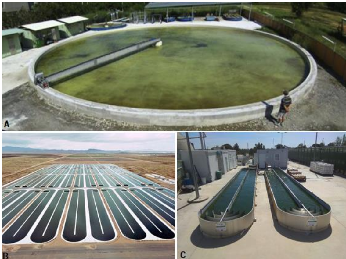
Figure 3 – Open systems for microalgae production. A: Circular pond located at the An-Nan campus, National Cheng Kung University, Taiwan (Chang et al., 2018); B: Raceways located in Qualitas farm, New Mexico (Nordrum, 2018); C: Raceway pilot scale installed in Allmicroalgae, Pataias, Portugal.
