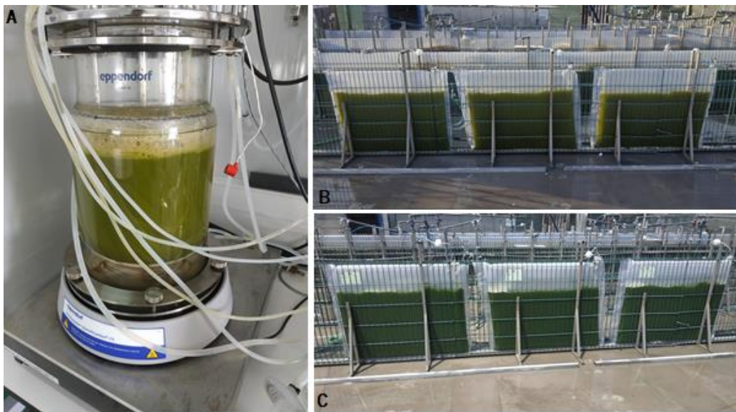
Figure 28 – Two stage cultivation. A: Organic Heterotrophic Inoculum. B: Three flat panels with same conditions after inoculation. C: Flat panels after 4 days of inoculation.
