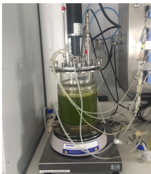
Figure 9 – 7 L bench-top fermenter (New Brunswick BioFlo®/CelliGen®115; Eppendorf AG, Hamburg, Germany) with organic medium.
