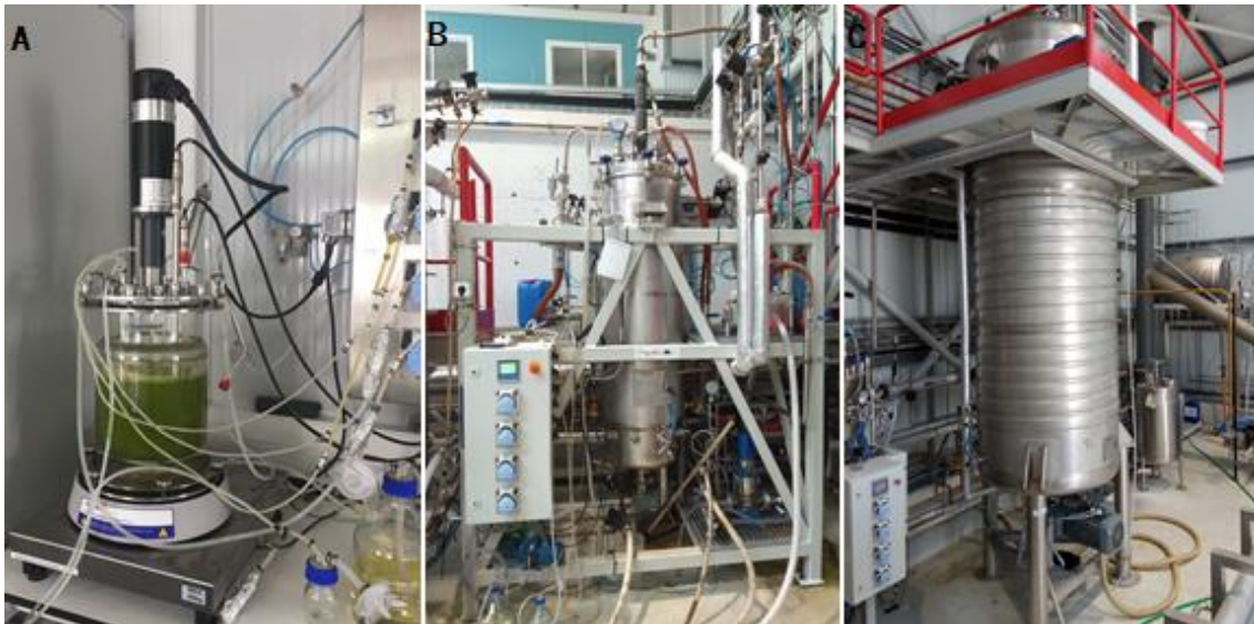
Figure 5— Fermenters with a working volume of: (A): 7L; (B): 200L; (C): 5000L. Pictures were kindly provided by Allmicroalgae, Pataias, Portugal.
