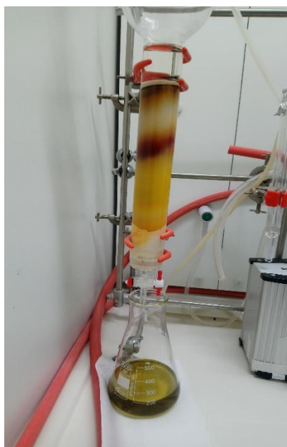
Figure 3.5. FC apparatus of FC of VLC fractions (GH) from Nodularia sp. LEGE 06071.
