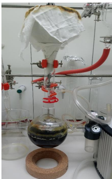
Figure 3.3. Extraction apparatus for organic extraction of Nodularia sp. LEGE 06071.
