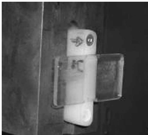
Figure 6. PET overmoulded onto a SL Huntsman 5260 block.
