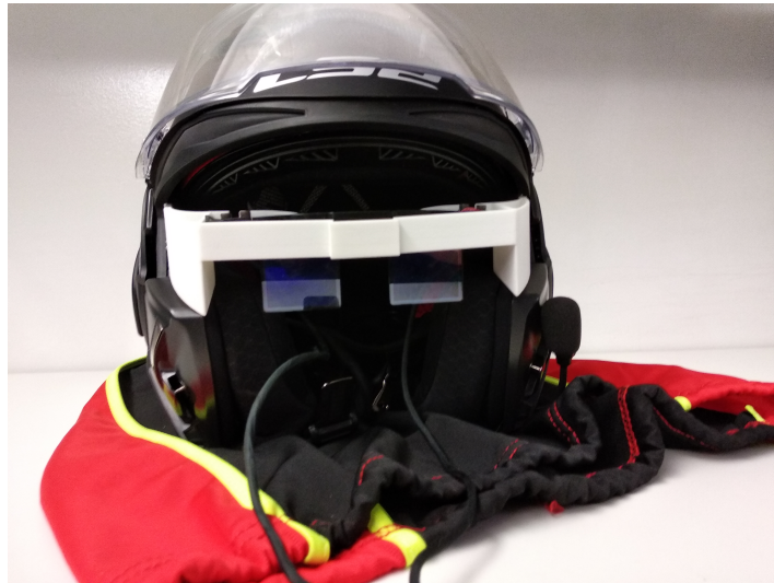
Figure 34: 3D printed mold with the smart glasses placed inside the helmet.
