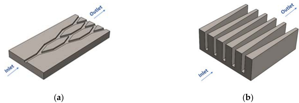
Figure 8. (a) Concept model of an enhanced surface with increasing cross-sectional area for a plane plate (b) and for a heat sink.
