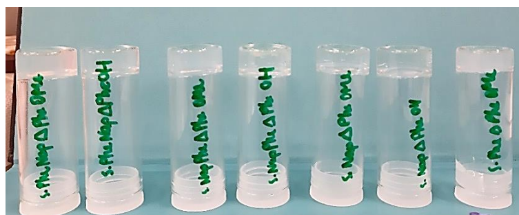
Figure 43 Inverted tube test for hydrogels at 0.4 wt % concentration (see Table 2). Order of the hydrogels, from left to right: 16, 17, 8, 9, 13, 14, 5.
