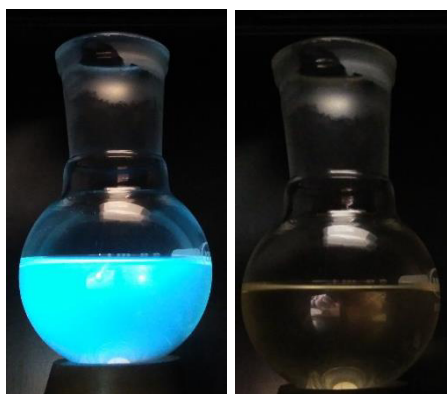
Img. 1. Solution compound 15d in DCM, under UV flashlight 325 nm (left), normal light (right)
