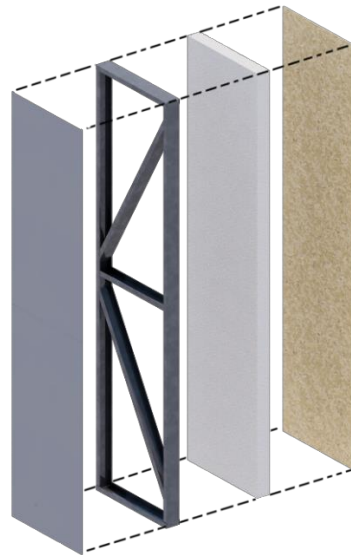
Figure 14 - LSF panel exploded view
