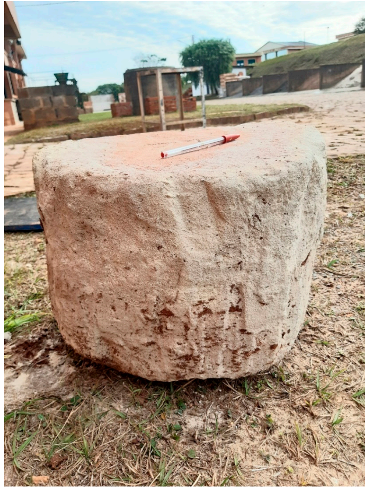
Figure 14. D_r 450 mm B_{SHS} stabilized layer exhumed from the soil.
