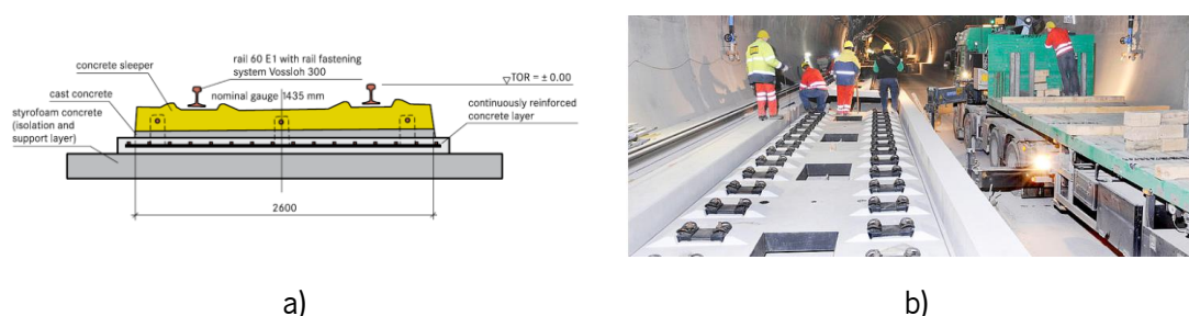
Figure 1.7 - Evolution/modifications of the ballastless tracks: a) Rheda system classic; b) Öbb Porr - prefabricated system
